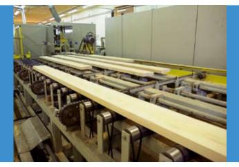
SMB's compact line is used especially in jointing larger dimensions for log-house manufacturing purposes.
