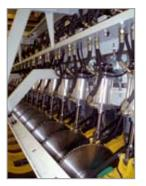
Cutting the green timber very accurately to the selling length allows to increase the green wood chips and thus to improve the productivity. One of the efficient cutting methods is trimmer sawing shown in the picture. For extremely high speeds we recommend the Jartek Free Cut system.
