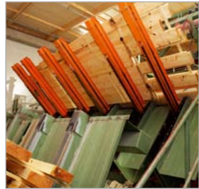
UNLOADING THE STICKERS: The pictures show the sticker unloading devices fitted with auxiliary unloaders. Thus the load change time is set to zero. Grading line for dry timber runs continuously and without any interruptions caused by the pile change.
