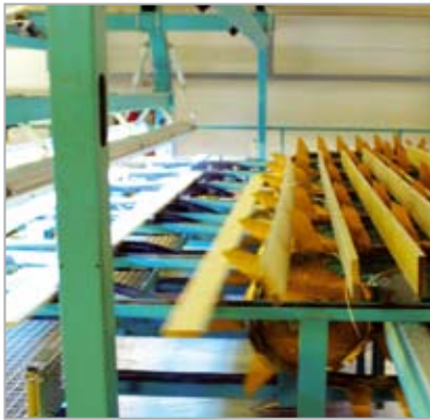
Automatic scanner grading, in between the pieces are turned.
