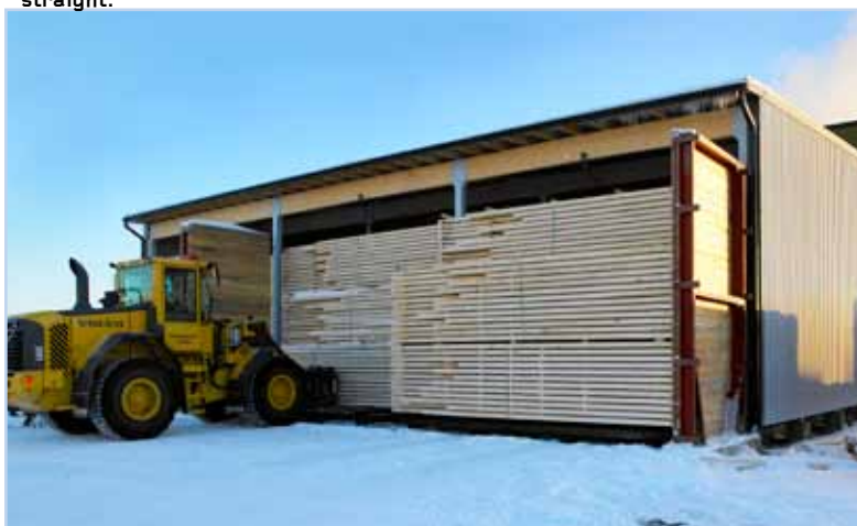
Kontiotuote, three two-stage compartment kilns, 40,000 m 3 /a
